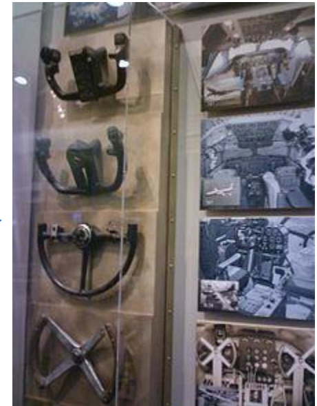
Collection of control yokes at Boeing Future of Flight Museum : 747, 707, B-29, Trimotor.
